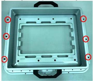
➤ Lift up the teflon module to check if glass have some residuals or dirt on it. Take out the glass & teflon tank assembly. (Refer following image)
