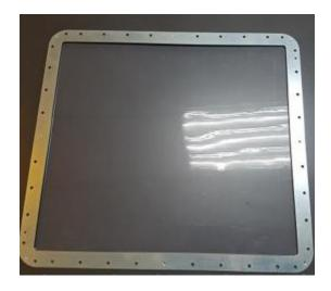
> Put the teflon film module on the tank surface & fit with pin position.
