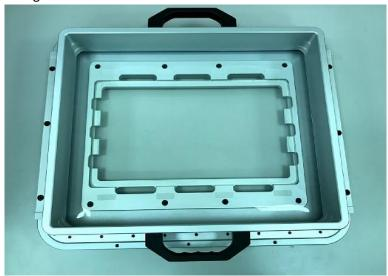
> Simply shift tank holder's 2 ribs at inner side & lock the 4 screws.
